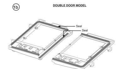
Remove the old rope and scrape old glue from the locating groove.
