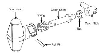
Check the door catch operation and tightness of the lock nut. Adjust if required.
