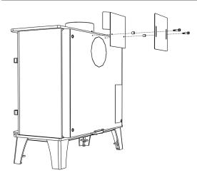
Align the Heat Shield on the slots to cover the gap between the Twin Wall and the Top Plate. The overlap must be at least 10mm.
