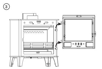
REMOVING THE DOOR - DOUBLE DOOR MODEL
