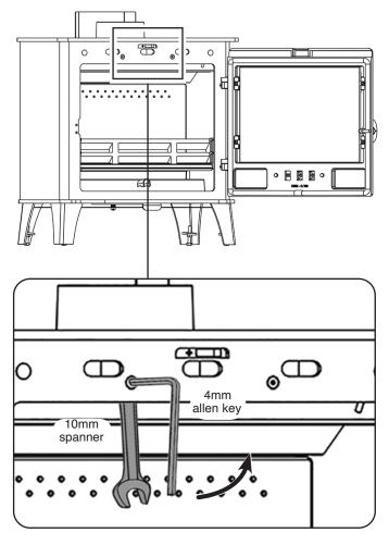
Loosen the hex bolt until the slider moves with no resistance. Once happy with the sliding action tighten the 2 locknuts.
